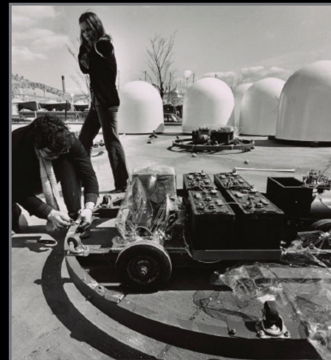
ART MEETS TECH: Artist Fujiko Nakaya and physicist Thomas Mee created artificial fog by spraying pure water through narrow nozzles installed on the Pepsi Pavilion's roof [above left]. The system tracked wind speed and direction [above right] to ensure the fog was distributed over the building's surface. On the pavilion's terrace, autonomous white “floats” built by sculptor Robert Breer [kneeling, below left] roamed about, emitting soft sounds [below right].
